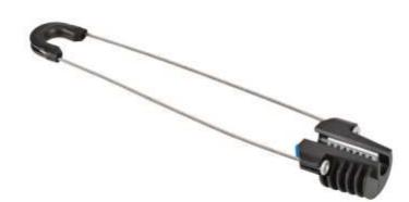
Designed for mounting and supporting the cable while ensuring the required tension of the cable line. Consists of open conical body frame, a pair of metal toothed wedges (clamping device) and a flexible bail. All parts are interconnected and cannot be lost. Installed in pairs at the beginning, at the end and in the interval of 5 supports along the length of the cable line. Provides a significant reduction in the duration of the cable suspension process.
