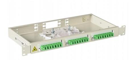
The SHKOS-L series cross optical rack is designed for installation in 19", 21", 23"racks. The cable is fastened to the sheath with a metal clamp and / or nylon ties, on a T-shaped petal. The central power element of optical cable is attached with a metal bracket. Interchangeable metal strips with 8 or 4 holes allow the installation of various types of socket adapters: FC, SC, ST, duplex LC.
