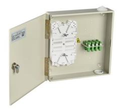
Wall-mounted crosses of the SHKON-U series are intended for placement in offices, control rooms, communication rooms and other serviced premises. The maximum capacity of SHKON-U crossovers is - 32 ports SC, FC or ST. When using LC connectors, the capacity is doubled. Optical cables are cut and fixed in the lead-in area. Further, the fibers in the modules go to cassettes for welding with pigtails. The adapters fit on 6 or 8 hole strips.
