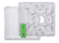
The cross socket (SHKON-PA-1) is designed for installation in offices and residential premises. The optical cable is laid and fixed on the base. The fiber is welded to the pigtail; splice protection kit is fixed in the stand. Fibrlok mechanical connectors can be used. The adapter is installed in one of the places on the base of the body frame.
