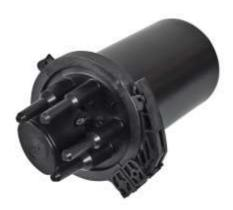
The dome closure MTOK-L7 is designed for the installation of self-supporting cable with a capacity of up to 48 optic fibers. An oval input allowed to accommodate a loop of optical loose tubes without cutting. The loop is laid out in the tray on the opposite side of the splice trays.
