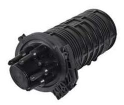
Dome closure MTOK-L6 is designed for the installation of self-supporting cable and urban cables of any design. An oval input allowed to accommodate a loop of optical loose tubes without cutting. The loop is laid out in the tray on the opposite side of the splice trays.
