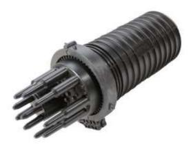
The dome closure MTOK-G3 is designed for the installation of self-supporting cable and urban cables of any design. An oval input allowed to accommodate a loop of optical loose tubes without cutting. The loop is laid out in the tray on the opposite side of the splice trays.
