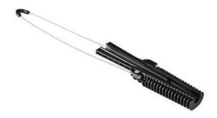
Designed for aerial installation of self-supporting cables like OKSN type. Consists of an open conic body frame reinforced with fiberglass, a pair of plastic wedges and a flexible stainless-steel bail of 250-500 mm.
